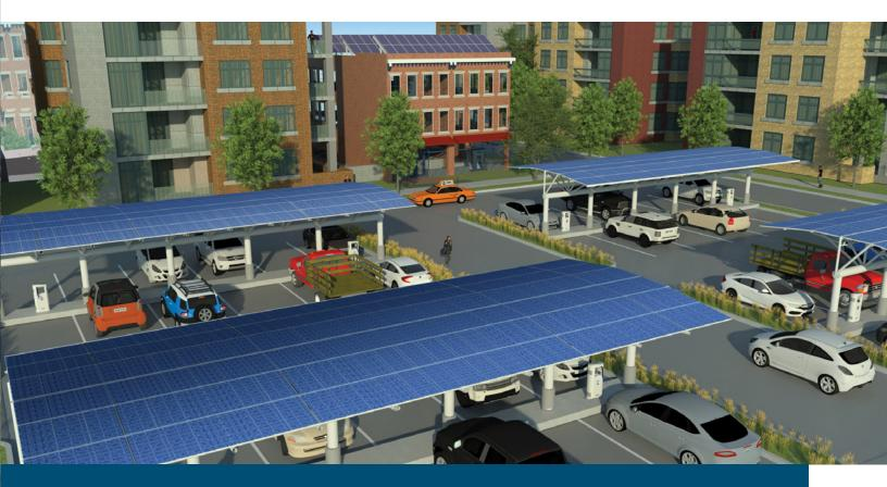
Parking lots and garages can offer ideal locations for solar installations because they often furnish the large, unshaded and unobstructed spaces optimal for such systems. Solar canopies in parking areas can provide shade and weather protection for cars parked beneath them as well as supply energy to electric vehicle-charging stations.
