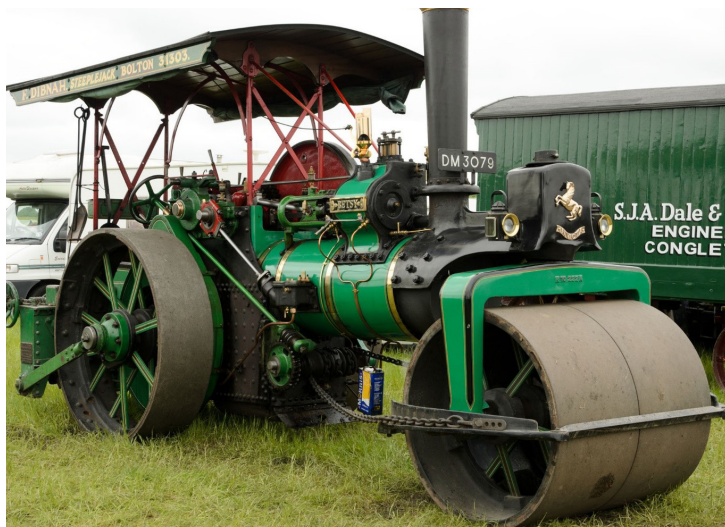
Example of a 1912 Road Roller used as the Live Load Design Vehicle (13 Tons) for most of the bridges. There are 11 ft. between the axles. The rear axle bears 8 tons and the front axle bears 5 tons.
