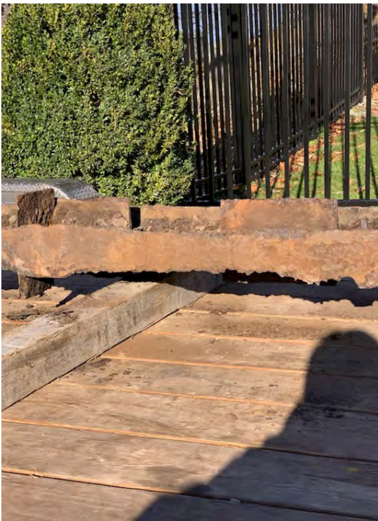
Corroded beam after removal
