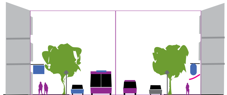
Diagram shows ratio of 1 building height to 2 road width.
