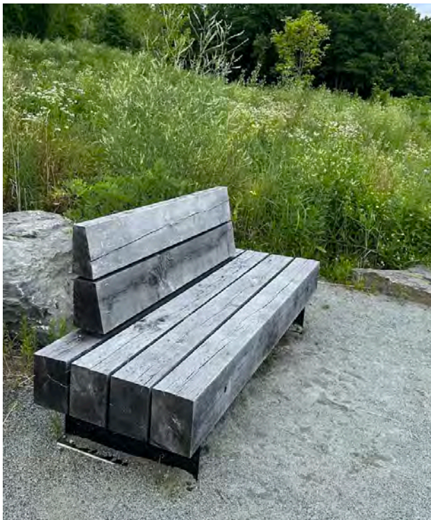
Figure 77. White oak and steel bench, Sojourner Truth State Park. Example of potential trail seating. Anchoring is not needed given the weight and can be installed on aggregate or concrete pad. Source: OLIN.
